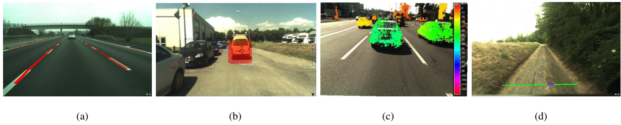
Fig. 2. Output from some of the systems installed on the vehicles: (a) lane detection, (b) preceding vehicle detection, (c) stereo obstacle detection, (d) ditch detection
