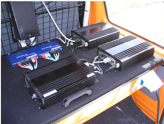
Fig. 5. The 3 onboard PCs installed into the booth of the first test vehicle.
