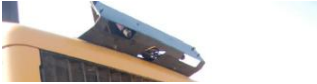
Fig. 2. Stereo cameras on the wheel loader hood
