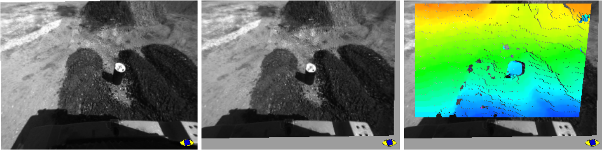
Fig. 3. Example of DSI engine processing: (a) left image, (b) right image (c) disparity depth map with the usual color coding. Note how the left and right images have been processed with rectification and lenses distortion removal procedure
