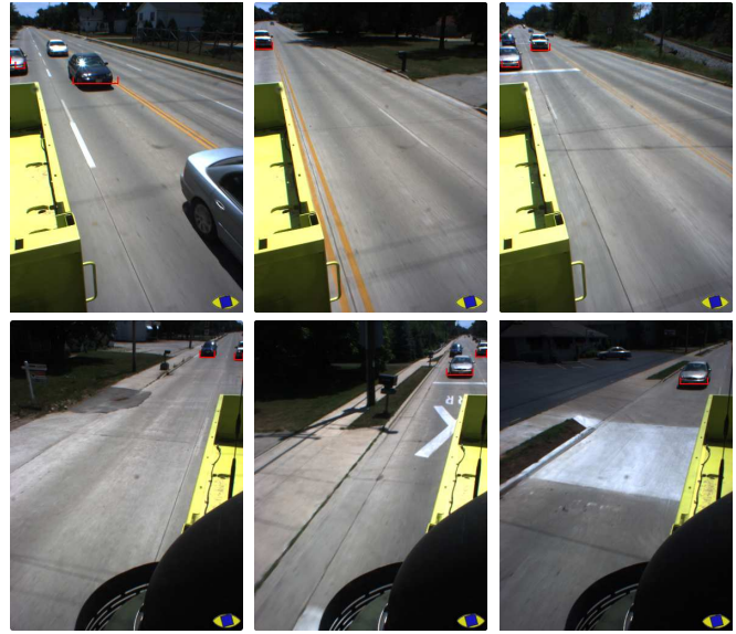
Fig. 8. Examples of Rear view output. In the upper row, images coming from the left side are shown, while those acquired on the right side are visible in the lower row. Overtaking vehicles are marked with a red line.
