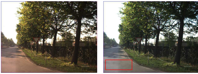
Fig. 5. Original image and result of chromatic equalization. In the right image the region supposed to frame the pave is shown.
