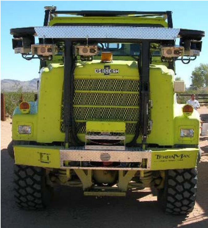
Figure 2: The TerraMax sensor suite: three cameras and two Sick LIDARs are installed on the rollbar; two IBEO Laserscanners are installed inside and over the front bumper; GPS antennas are visible on top of the vehicle's roof
