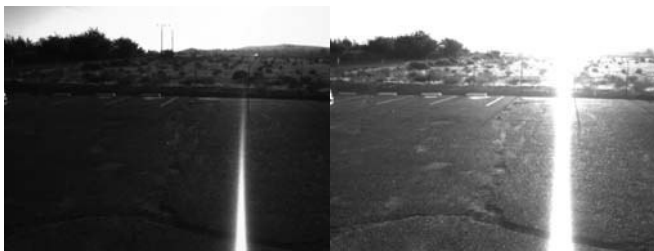
Figure 5: Image representing the view without and with the developed camera gain control scheme; in the right image, although a part of the image is oversaturated, the terrain is visible and the algorithms for obstacle and path detection can be run
