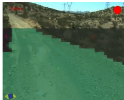
Figure 4: the result of path detection in green; the red dot in the top right corner represents the status of the 'straight-road'-detection: in this case 'red' means curved road.
