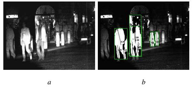
Fig. 10. Worst case: original input image (a) and respective output one (b) with detected objects main axes of minimum inertia and surrounding bounding boxes visualized; the green bounding box highlights the only pedestrian detected.
