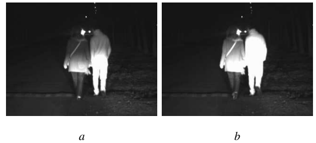
Fig. 2. Employment of dipped-beam (a) and full-beam (b) headlights.
