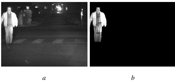
Fig. 9. Best case: original input image (a) and respective output one (b) with pedestrian's main axes of minimum inertia visualized on it.
