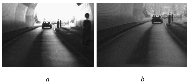
Fig. 13. NIR images acquired with a CCD (a) and a CMOS (b) camera.
