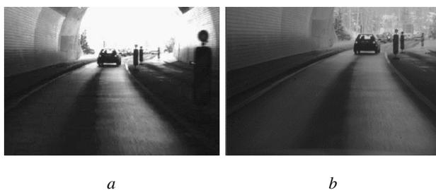
Fig. 13. NIR images acquired with a CCD (a) and a CMOS (b) camera.
