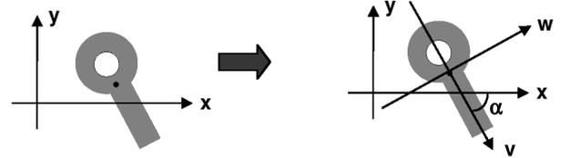
Fig. 4. Axis of minimum inertia for a generic object.
