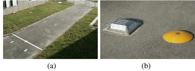
Fig. 1. Vision system calibration: (a) stretch of road used for the vision system calibration equipped with (a) near and far IR markers.
