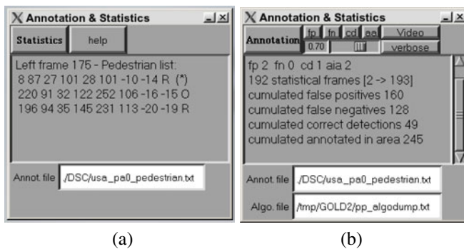
Fig. 6. (a) Statistics extraction screen-shot: for each frame values of CD, FP, FN are computed and cumulated up to the current frame. (b) Annotation panel during the human supervised annotation process: information about current operation are displayed
