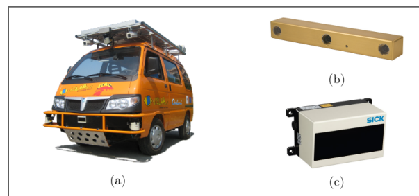
Fig. 1: The recording platform. Data has been collected using one of the electric vans a) which had been set up in 2010 to take part to the VisLab Intercontinental Autonomous Challenge (VIAC) [7]. b) The imaging unit is synchronized to a LIDAR c) working at a frequency of 12.5 Hz.
