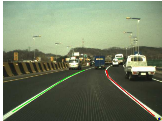
Figure 3: Algorithm output and processing images: IPM image (top left), candidate polylines (top center) and detected lane markings (top right); original image with detected lane markings superimposed (bottom).
