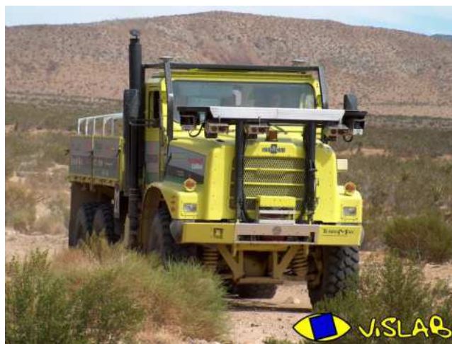
Fig. 1. The TerraMax vehicle. Two ALASCA laserscanners are visible above and inside the front bumper, the three cameras and the two SICKS are placed on the bar over the hood.
