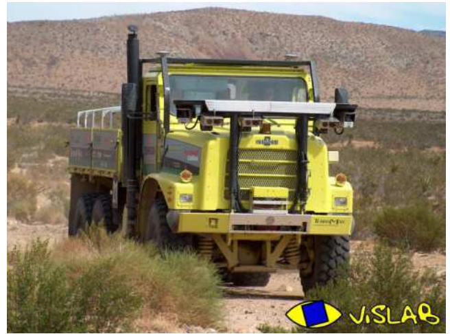
Fig. 1. The TerraMax vehicle. Two ALASCA laserscanners are visible above and inside the front bumper, the three cameras and the two SICKS are placed on the bar over the hood.
