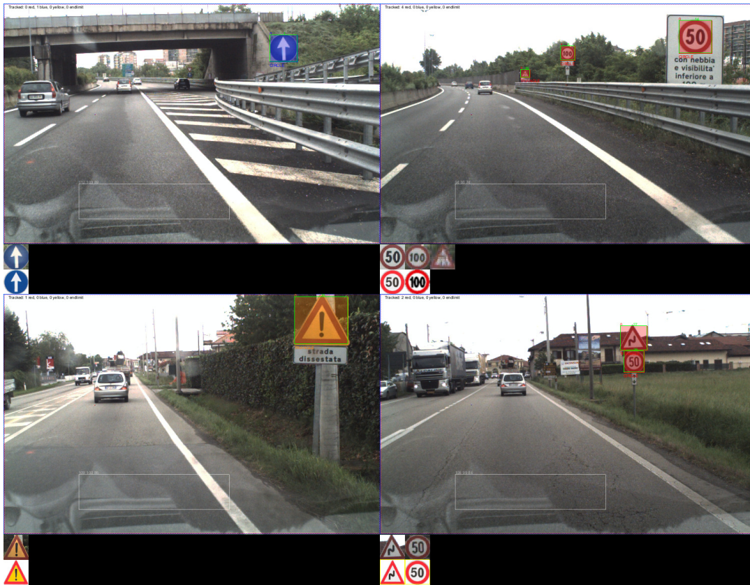
Fig. 14. Example of system results in different environment and light conditions. In the bottom part of images the first row shows regions provided by detection stage and the second the output of classification
