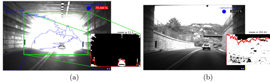
Fig. 6. Exit from a tunnel. (a) Filtered and binarized bounding box before the tunnel exit, (b) filtered and binarized bounding box after the tunnel exit.
