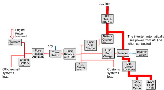
Fig. 6. Electrical System block diagram.
