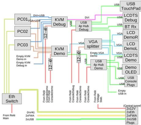
Fig. 4. Hardware and connections of the console layer.
