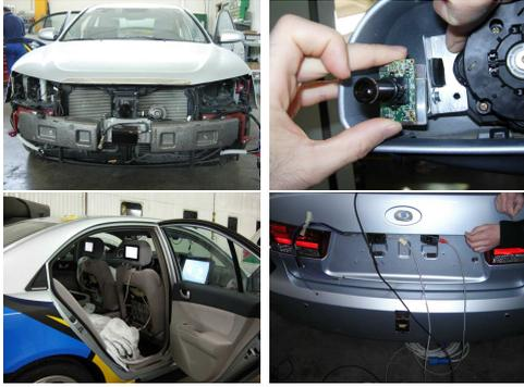
Fig. 5. The Lux laser installed on the front bumper's center with the IDIS one on top of it (top left); mirror camera mounting (top right); inside view of the car (bottom left); stereo camera system and UTM-30LX laser installed on the back side (bottom right).
