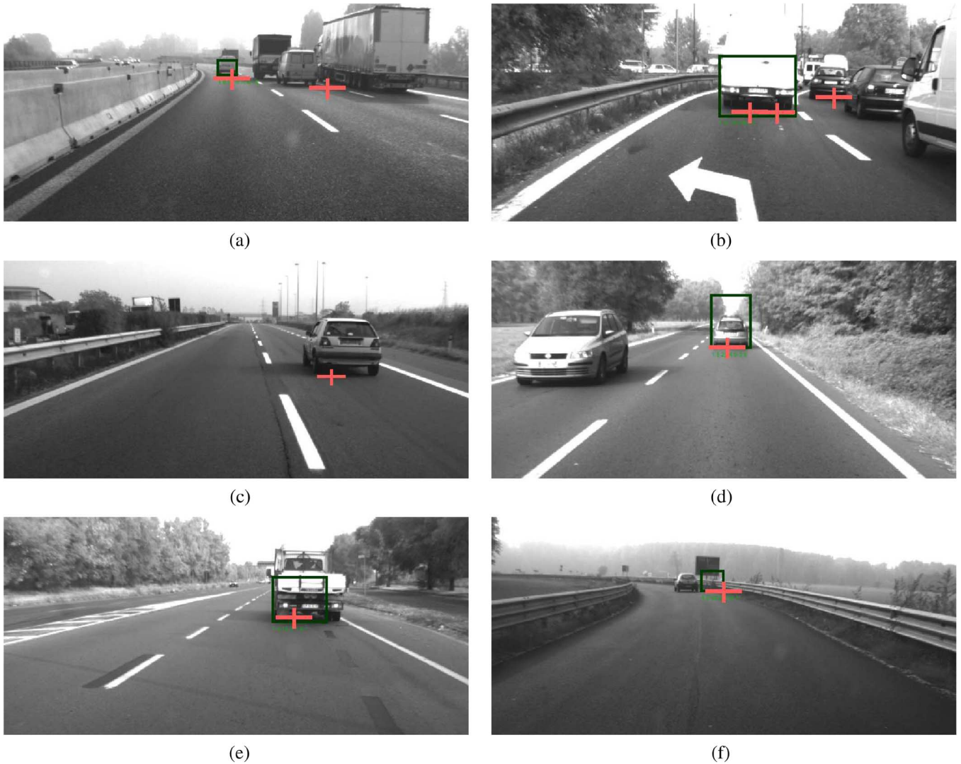
Fig. 19. Examples of errors. (a) and (b) The most frequent errors are due to traffic, but some errors may also happen in simple cases. (c) A vision false negative due to low contrast on the left border. (d) A radar false negative (the oncoming vehicle). (e) An inaccurate detection. (f) A false positive due both to vision and the radar.
