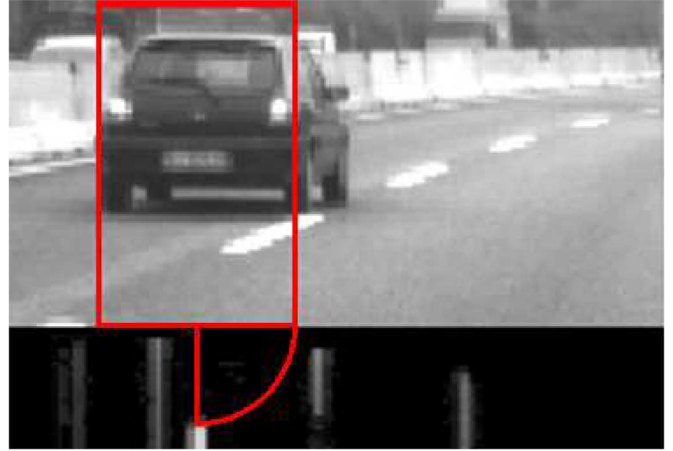
Fig. 8. Box width computed from peak height.
