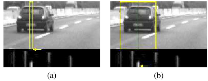
Fig. 5. Symmetry computation. Arrows indicate where the symmetry value is stored for (a) a single column width and (b) the largest width. Symmetry is computed in the area enclosed in the bright rectangle and using the dark vertical line as an axis.
