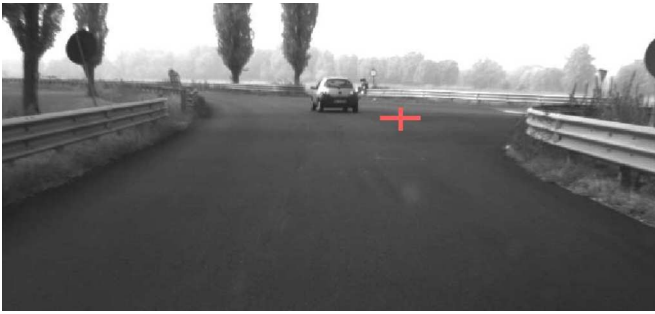
Fig. 4. Lateral radar error. The radar data falls outside of the object shape.
