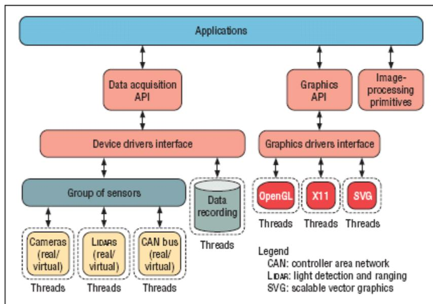
Fig 12. The GOLD architecture. The different colors represent software blocks belonging to same logical level.
