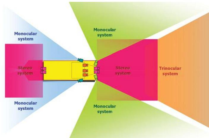
Fig. 6. Vision coverage of TerraMax (truck facing right). Systems displayed: Trinocular (orange) looking forward from 7 to 40 m, stereo front and stereo back (purple) monitoring a 10×10 m area on the front of the truck and 7×5 m in the back, Rearview (blue) monitoring up to 50 m behind the truck, and lateral (green) looking up to 130 m.
