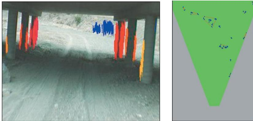
Fig. 12. Obstacle detection: the color of the obstacles varies with distance. The image on the right maps the obstacles in a bird's eye view. The camera's field of view is plotted in green.
