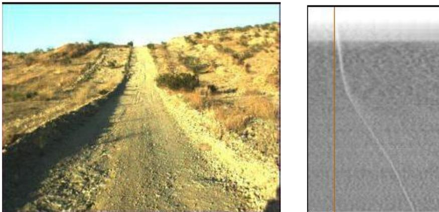
Fig. 9. V-Disparity image analysis in a non flat ground scene.
