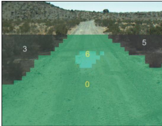
Fig. 10. White numbers denote off-road clusters, and yellow numbers denote road clusters. The interest area is limited to the region within 50 meters from the vehicle. This information is obtained from the preliminary processing of the obstacle-detection module.
