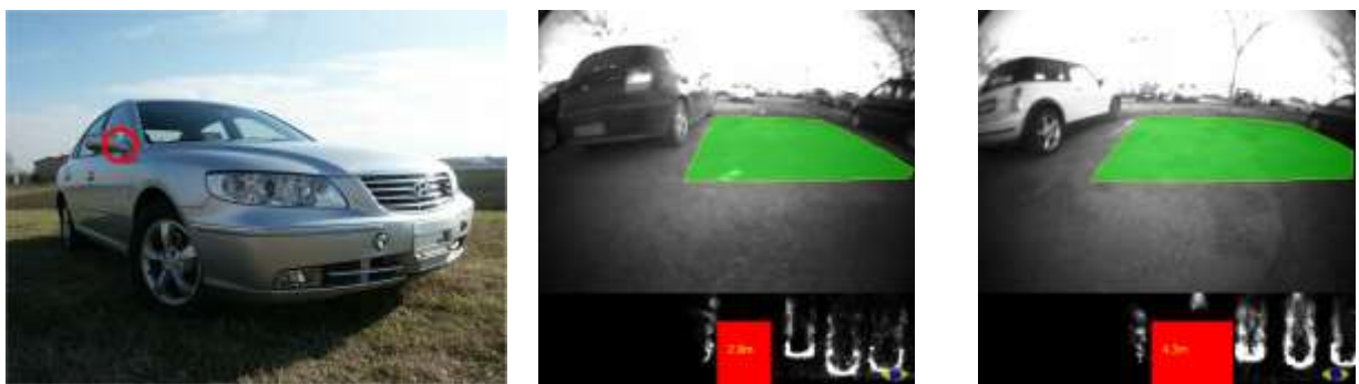
Fig. 7 The Hyundai Grandeur had a single b/w camera installed near the wing mirrors for parking assistance purposes; both images on the right show examples of free space detections: green areas (red in the bird's eye view underneath) are suitable for parking the car
