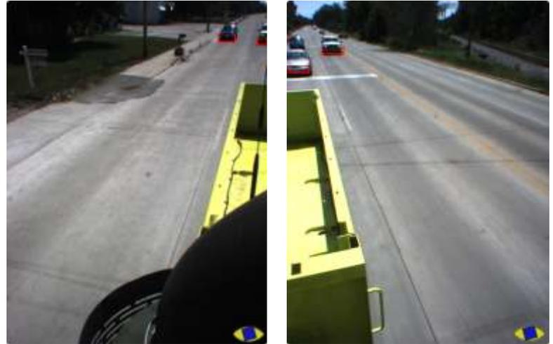
**Fig. 8** TerraMax T2 rear view system consisted of 2 color cameras placed on top of the truck cabin, pointing backwards [2]; right images show some approaching cars detected by red U-shaped lines
