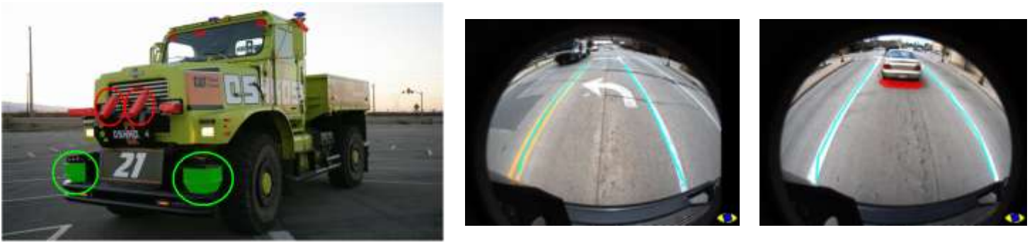
Fig. 10 TerraMax T2 frontal system for near obstacles detection consisted of a color cameras stereo pair and 2 laserscanners (described in Fig. 2.1 caption) [2]; the right images roadway lanes and a preceding car being correctly detected
