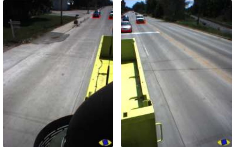
Fig. 8 TerraMax T2 rear view system consisted of 2 color cameras placed on top of the truck cabin, pointing backwards [2]; right images show some approaching cars detected by red U-shaped lines
