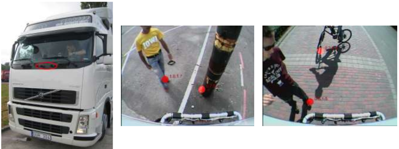
Fig. 11 Another color cameras stereo system installed by VisLab on the front of a Volvo truck cabin, for near obstacles detection [6]; examples of the system's output are shown in the right image
