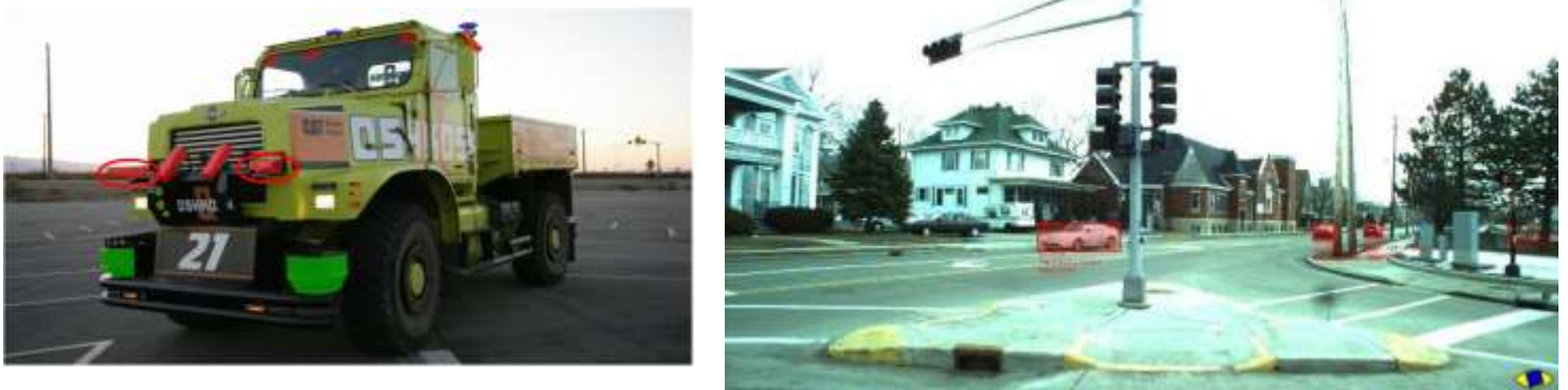
Fig. 6 TerraMax T2 was equipped with a lateral system made of 2 color cameras placed on a bar in front of the ventilation grid with the purpose of detecting cars approaching at traffic junctions [2]; right image shows an output example of T2 lateral system: cars driving towards the junction are framed by a red bounding box
