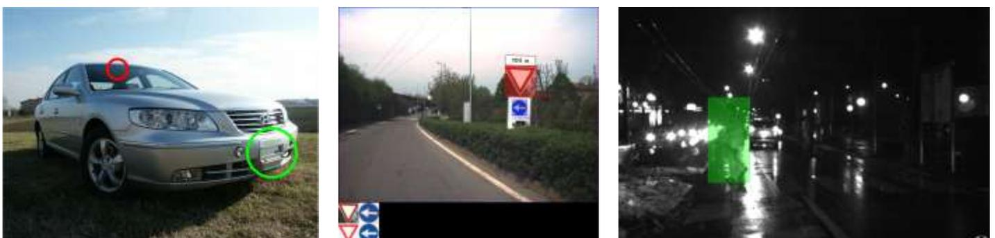
**Fig. 4** The Hyundai Grandeur had a single b/w camera installed behind the windscreen and a laserscanner with a 90 degrees scanning range and an extended sensing range up to 80 meters to detect road signs [5] and pedestrians [3]; images on the right give some examples of its outputs: road signs detection and pedestrian detection during nighttime visibility conditions
