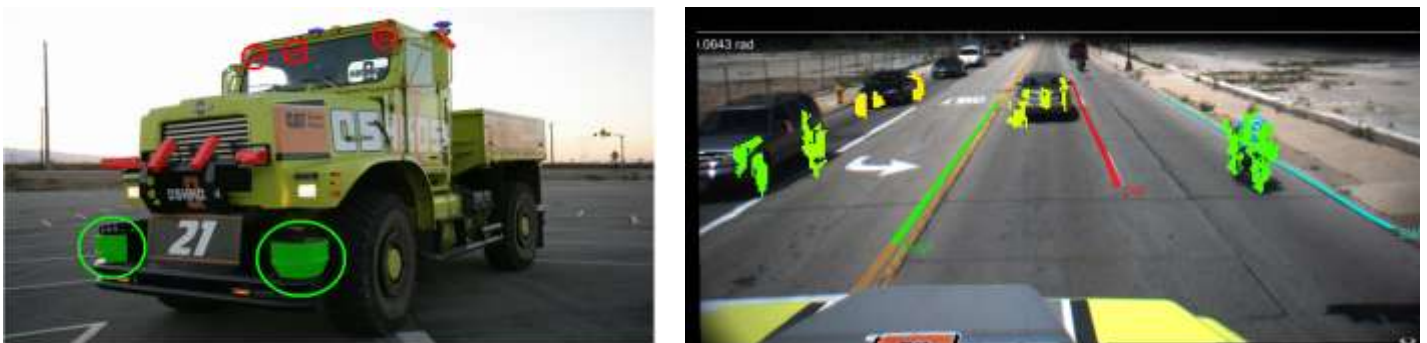
Fig. 3 TerraMax T2 head-on area was equipped with a trinocular color cameras system and 2 laserscanners for obstacles and lane detection [2]: system output is shown in the right image
