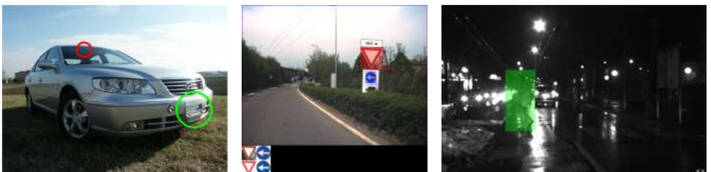
Fig. 4 The Hyundai Grandeur had a single b/w camera installed behind the windscreen and a laserscanner with a 90 degrees scanning range and an extended sensing range up to 80 meters to detect road signs [5] and pedestrians [3]; images on the right give some examples of its outputs: road signs detection and pedestrian detection during nighttime visibility conditions
